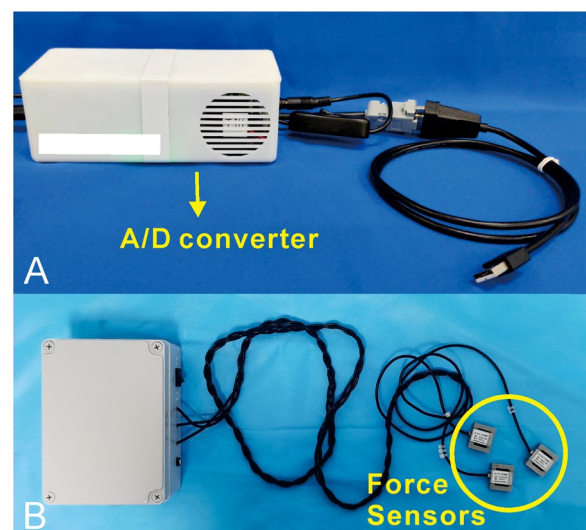
Fig. 2 Force collecting devices. a Custom-made A/D converter. b Three dismountable force sensors for measuring the force carried by the fixator
