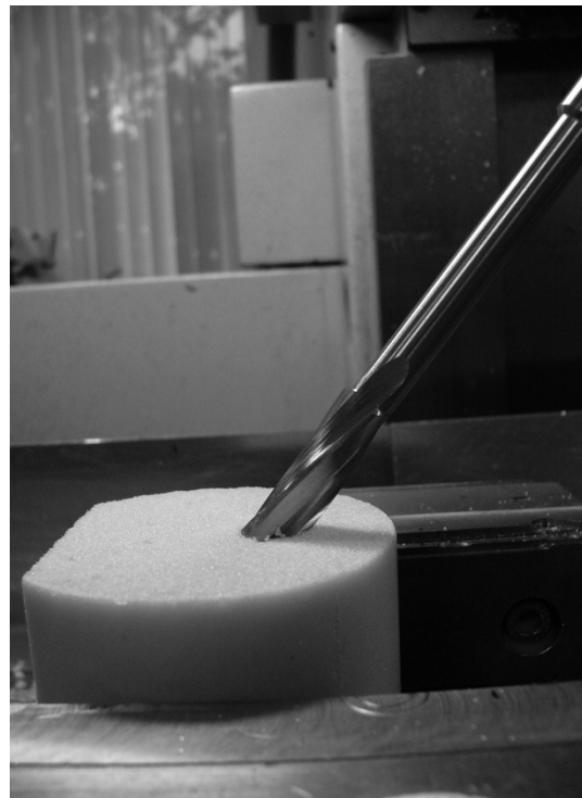
Fig. 5. Three-graded drill (TGN and Gamma 3).
